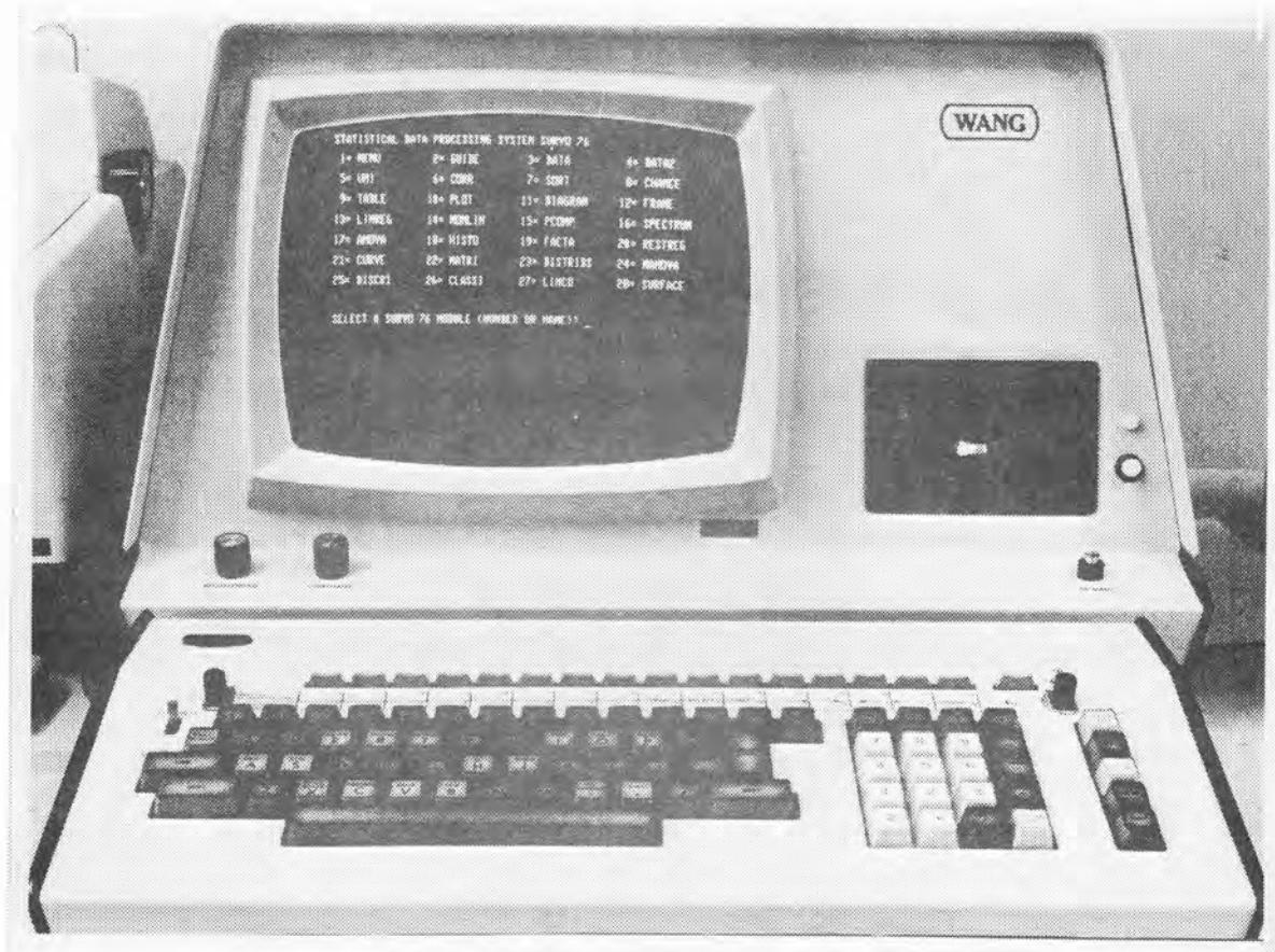
Fig. 1. The CRT display and keyboard of Wang 2200.
